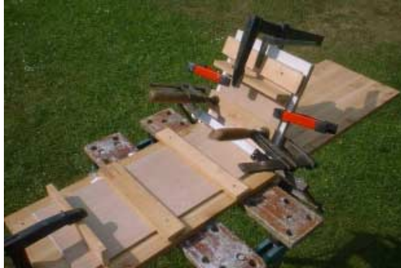
Figure 17: The seat jig with the two veneers mounted.
