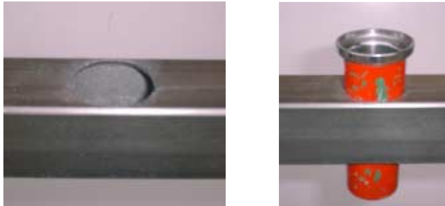
Figure 6: The hole for the head tube, and the head tube mounted in the square tube.
