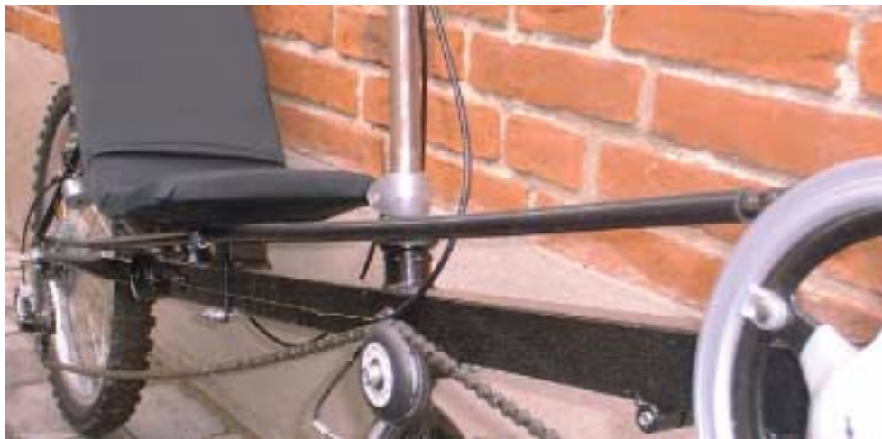
Figure 27: Chain tube made out of “plastic garden watering system tube”
