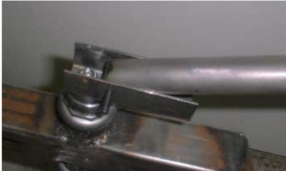
Figure 22: One implementation of adjustable over seat steering.
