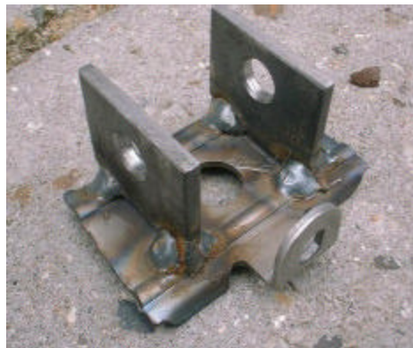
Figure 15: Spring mount after welding.
