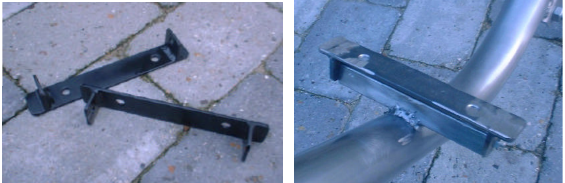
Figure 33: Seat mount solution 1 after welding and painting.
