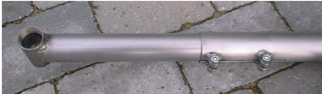
Figure 39: The pedal mount attached to the main tube.
