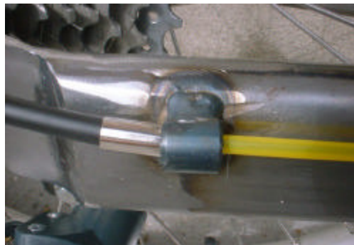
Figure 40: Two cablestops at the rear fork.
