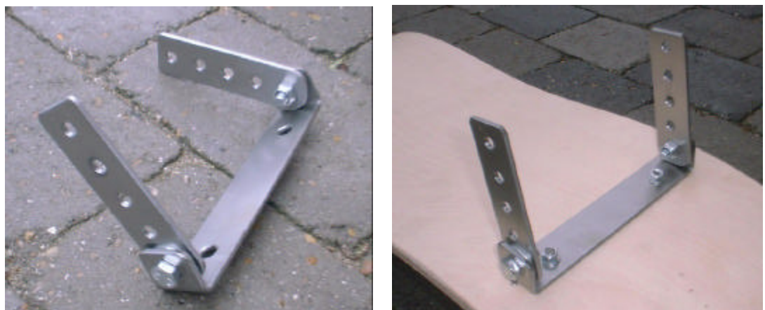
Figure 34: Seat mount solution 2 before paint.
