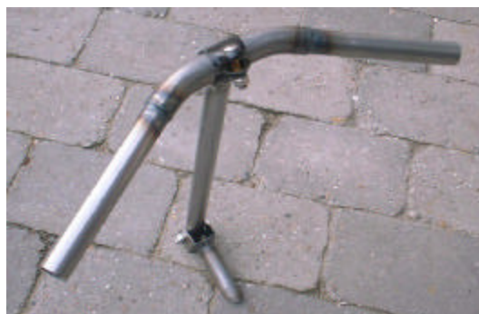
Figure 29: The complete stear after welding and the stem alone
