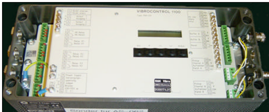
Figure 45 –photo du module "Vibrocontrol" (Bruel & Kjaer)
