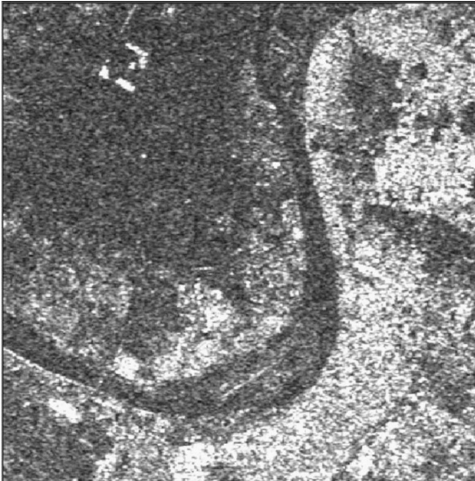
Fig. 3. SIR-B scene for Wad Medani, Sudan, collected in November 1984. Scene width is approximately 10 km. The river can be seen as a meandering low backscatter feature across the frame. Along the river and to the east and south are high backscatters from the urban and vegetative features. The low backscatter to the northwest is flat, bare soil acting as a specular feature.
